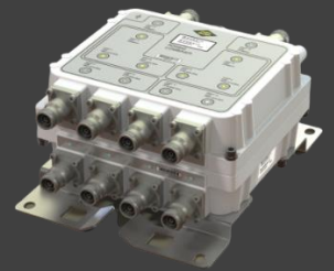
RD0842: 1400 / 1800 – 2600 MHz 4x4 Combiner with Auto Bypass™
